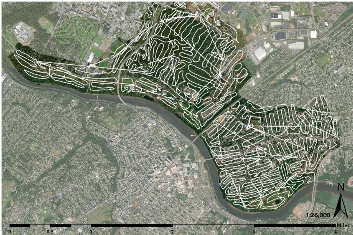
Figure 1. sUAS flight mission paths indicating extent of spatial coverage in search area in Highland Park, Rutgers EcoPreserve and Johnson Park in 2019
